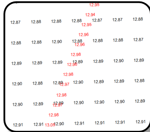
Figure 8. SBES and MBES data comparison at reference surface.
