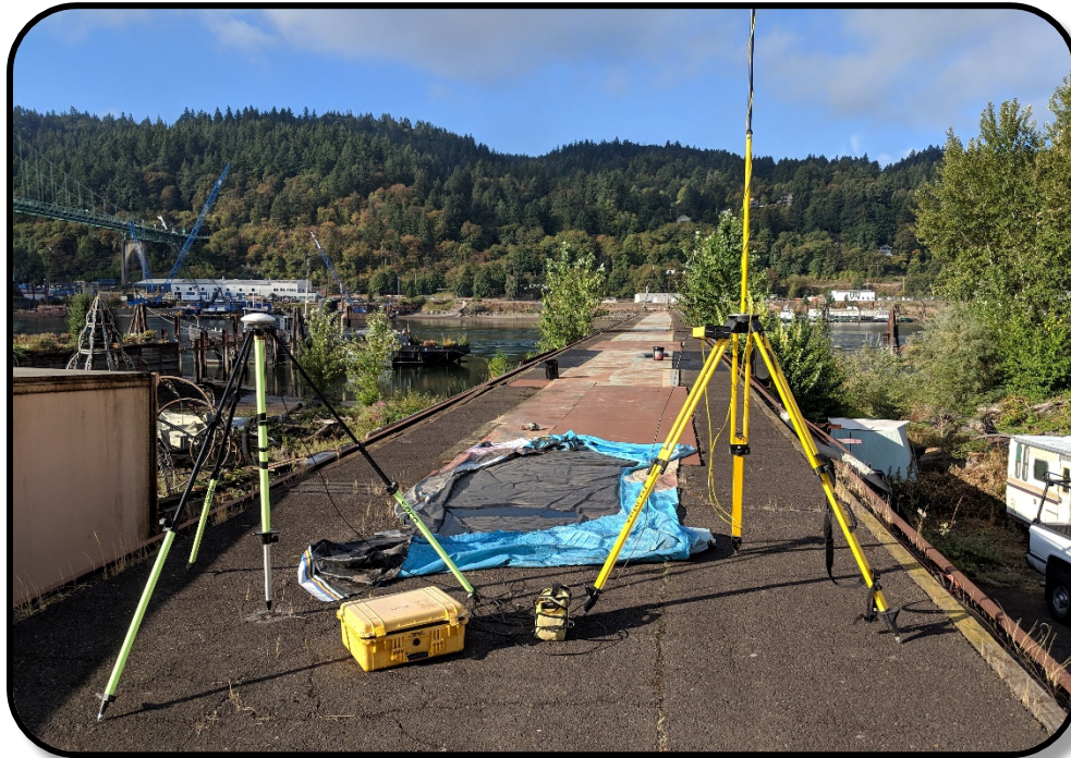
Figure 3. RTK GNSS base station and radio setup at SHI-1.
