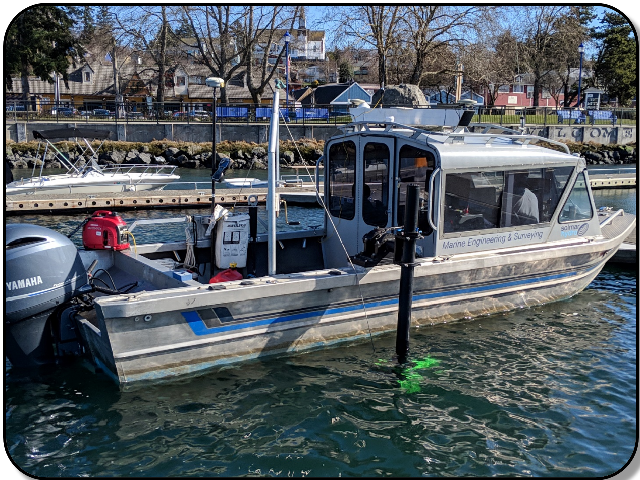
Figure 2. SHI's shallow water 24' survey vessel with multi-beam sonar in water (on side pole mount)
